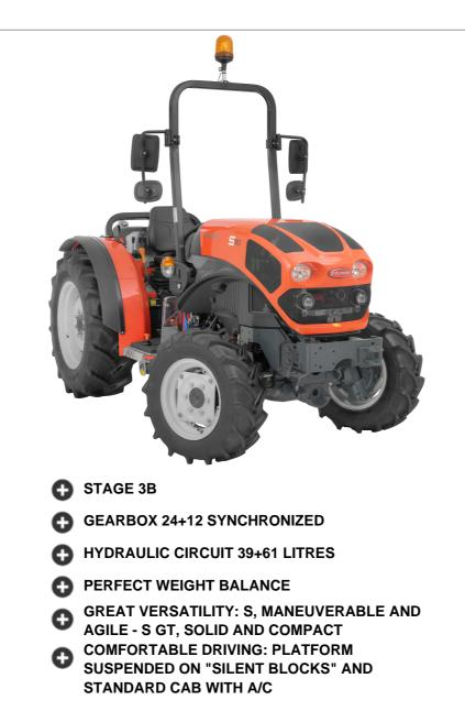
A "little" machine for orchards and vineyards with more than 100 horsepower? The S series (turbo intercooler, four-wheel drive, platform mounted on silent-blocks and a cab with a 360-degree view and air conditioning) will give you no cause to wish for a larger tractor. Balanced, compact, tough and tireless, these are the ideal companions for working worry-free, and there are 6 versions, so that you can find one that EXACTLY suits your needs.
