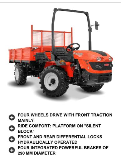
Goldoni Transcar range has been designed to meet the specific needs of people who work in mountainous areas and require a machine that's particularly suitable for materials handling. With 38 to 71 hp, air or water cooled engines to choose from, steering wheels or articulated versions, 2 homologated versions available such as agricultural tractor or as utility vehicle.
